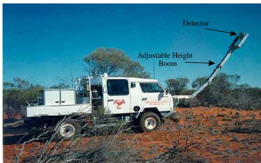
Figure 2. OKA vehicle with area-averaging gamma-ray system
