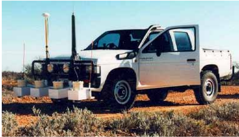
Figure 3. Nissan vehicle-mounted particle detection system
