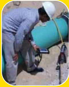
Industrial radiography of pipes using Iridium-192
