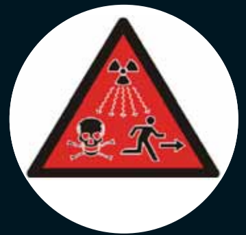
Example of new supplementary warning sign for category 1 and 2 sources
