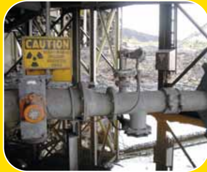
Industrial gauges containing radioactive sources installed on pipes for process measurements
