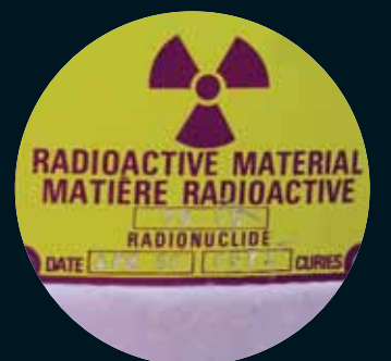
Example of radiation device label showing type of radionuclide, activity and date
