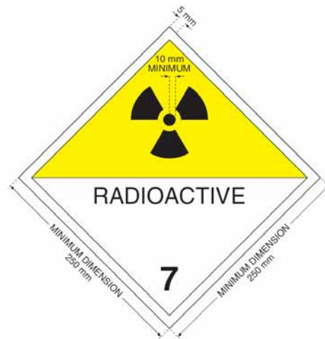
Figure 2 Placard for vehicle or freight container
