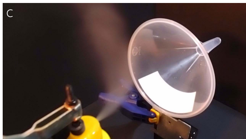
Figure 7. Observations during the cross-wind experiments. A) Sunscreen projected out of the aerosol product in a straight line when no wind was present. B) When wind was applied at a velocity at of 10 kph the sunscreen was blown slightly sideways. C) When wind was applied at a velocity at of 20 kph the sunscreen was blown sideways.
