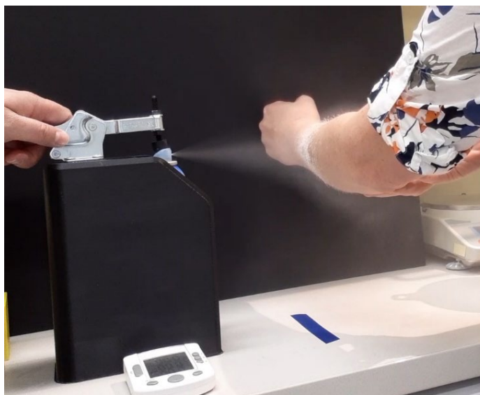
Figure 2. The actuator device. The calibrated actuator device dispersing a jet-spray of sunscreen onto an arm 10cm away from the bottle.
