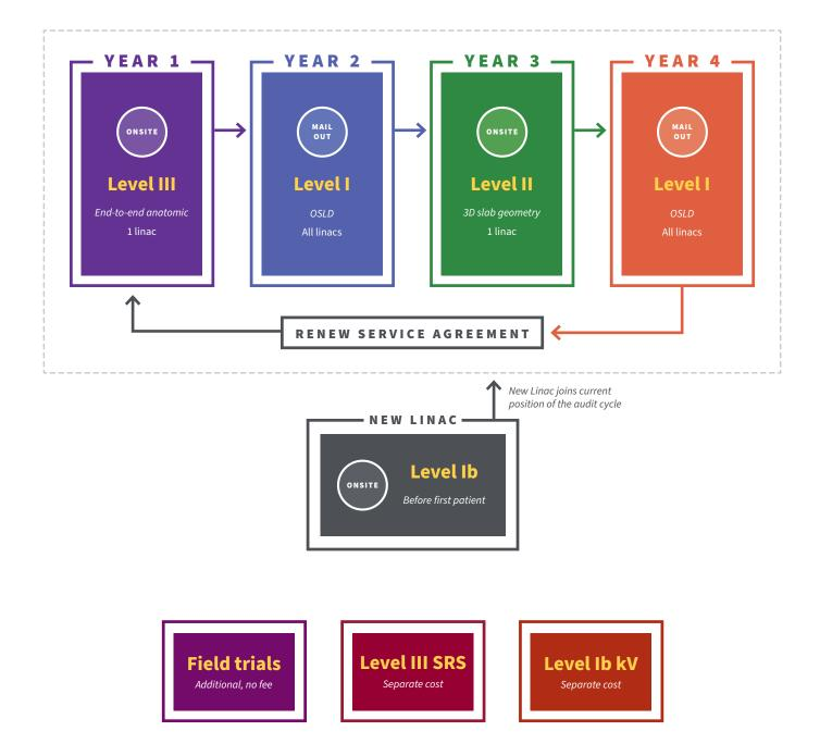
The current audit program includes Level I, Level Ib, Level II and Level III audits. Each Level II and III audit consists of various cases representing standard tests and clinical cases that sample a limited yet challenging set of complex treatment scenarios.
