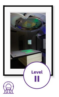
Array measurements in a slab phantom geometry to test TPS performance
