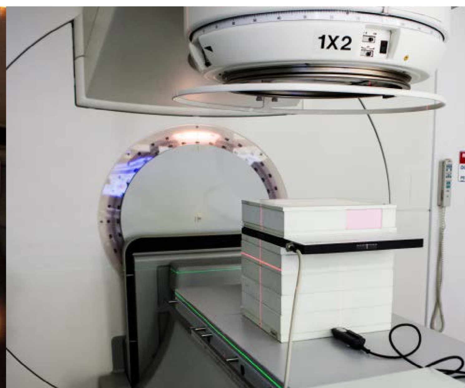
Figure 1c: The Level II audit uses a PTW 729 array with Computerized Imaging Reference Systems, CIRS, plastic water and synthetic lung.
