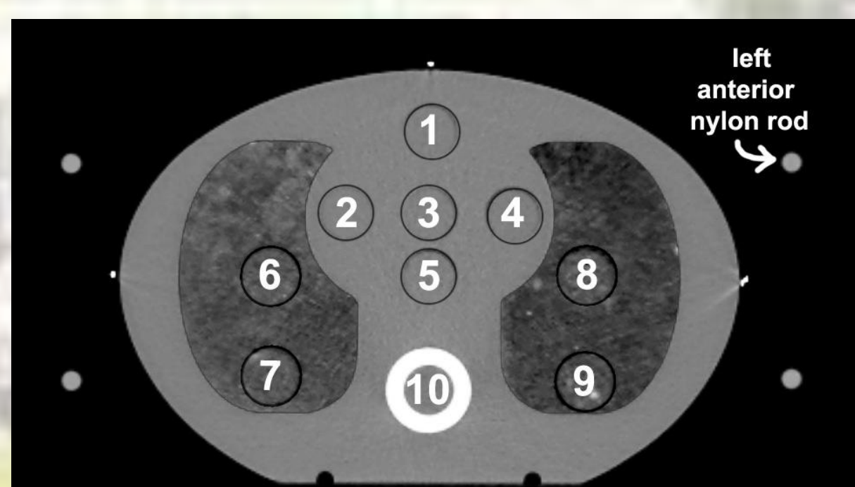
Figure 1: CIRS thorax phantom. CT image and phantom setup for measurement at linear accelerator
