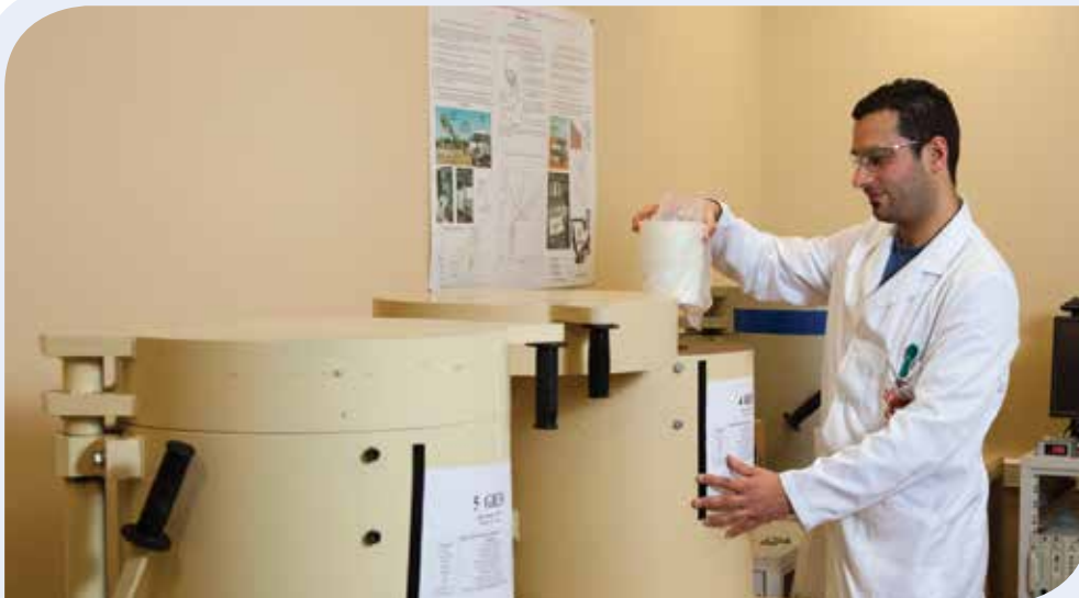
ARPANSA radiochemist placing a food sample into the Germanium Gamma Ray spectrometer to measure radioactivity.
