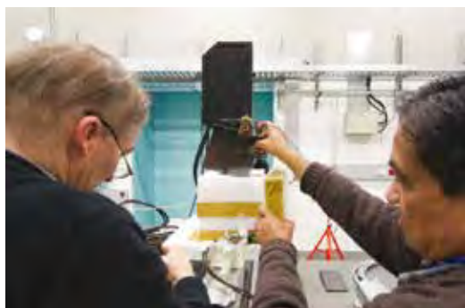
Staff from ARPANSA's Medical Radiation Services Branch at the Australian Synchrotron in Clayton, Melbourne at work positioning the graphite calorimeter inside a polystyrene box for thermal insulation
