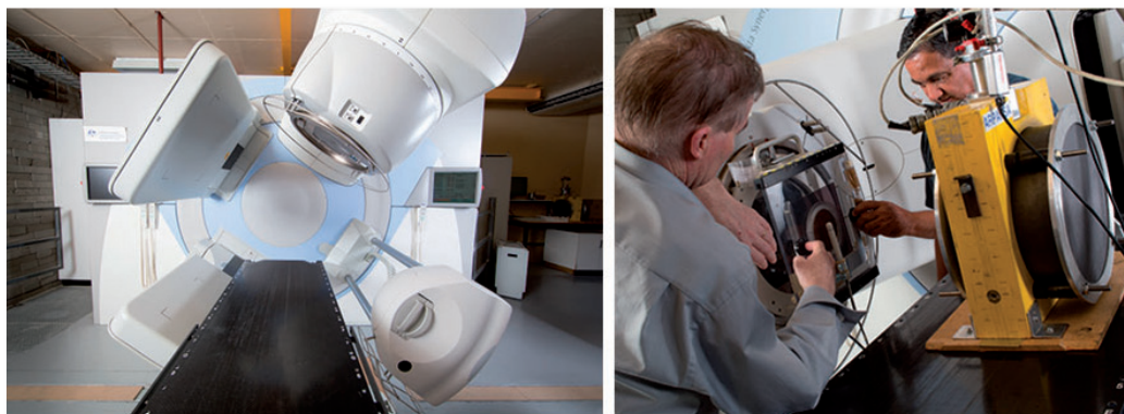
(Left) The linac at ARPANSA with which new calibrations services have been developed. (Right) Staff from the Medical Radiation Services staff setting up the primary standard graphite calorimeter on the linac.
