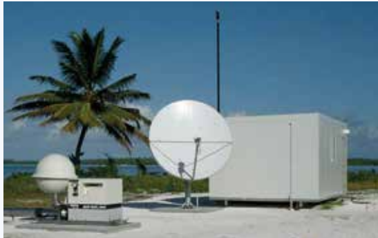
The Radionuclide Monitoring Station on Cocos (Keeling) Island. Particulate matter from the air is collected on a filter using the high-volume sampler at the left of the compound. The radioactivity collected on the filter over a 24-hour period is measured using highly sensitive instruments inside the building at the right of the compound. The results of the measurement are transmitted to the CTBT Data Centre in Vienna via the satellite dish in the centre of the compound.
