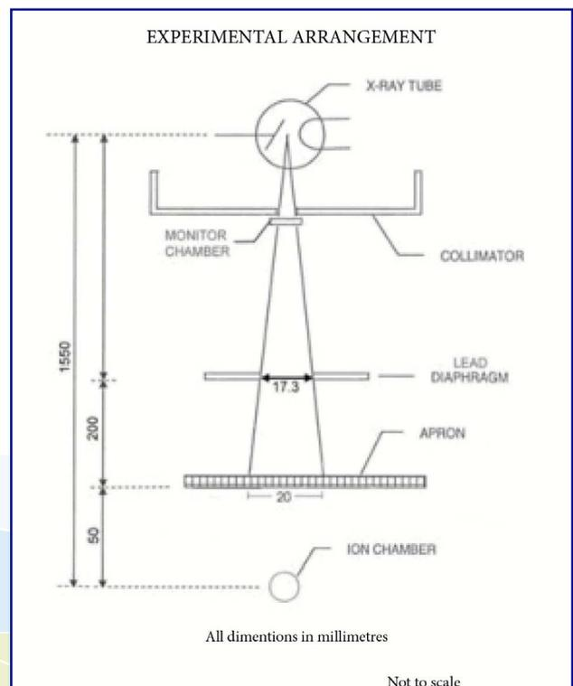
Measurements are made either with IEC/AS standard beams or common beams in clinical use.
