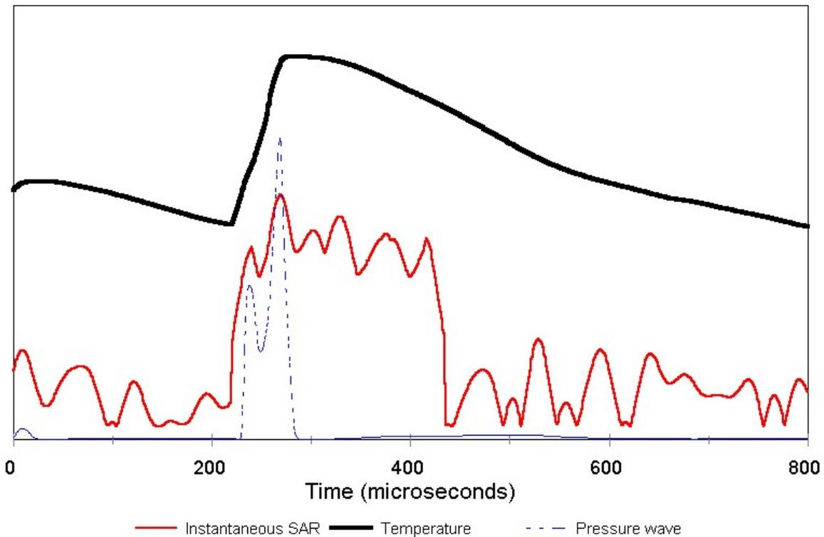
**Figure 1** Simulated temperature and pressure waveforms associated with arbitrary localised SAR waveform
