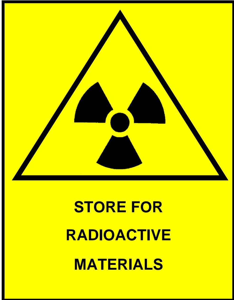
**D4 EXAMPLE OF A SUITABLE WARNING LABEL FOR ATTACHMENT TO A FIXED RADIATION GAUGE CONTAINING A RADIOACTIVE SOURCE**
