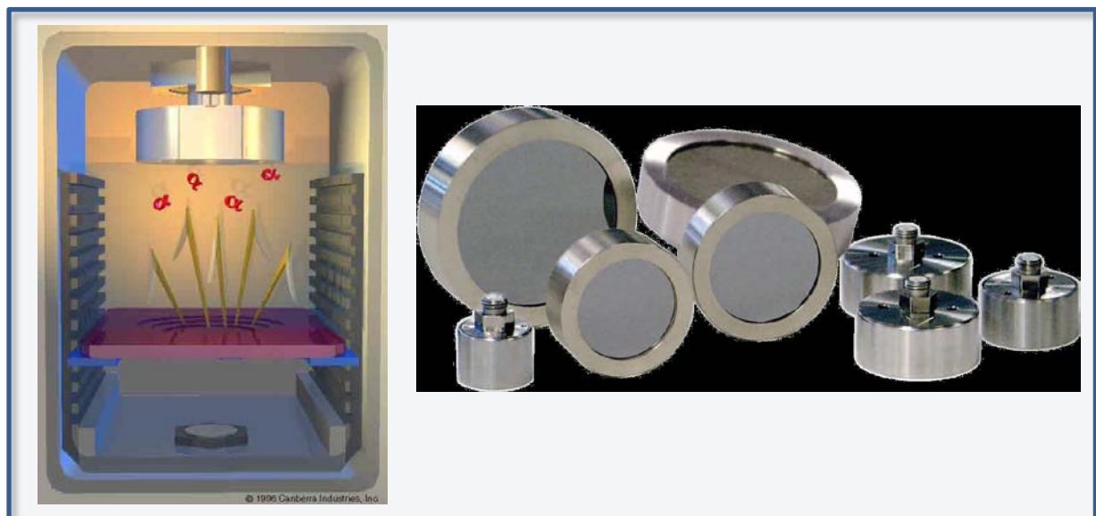
Figure 1: The arrangement of detector (silver) and source holder (red) in an alpha-spectrometry chamber (left) and the detectors used for alpha-spectrometry (right).
