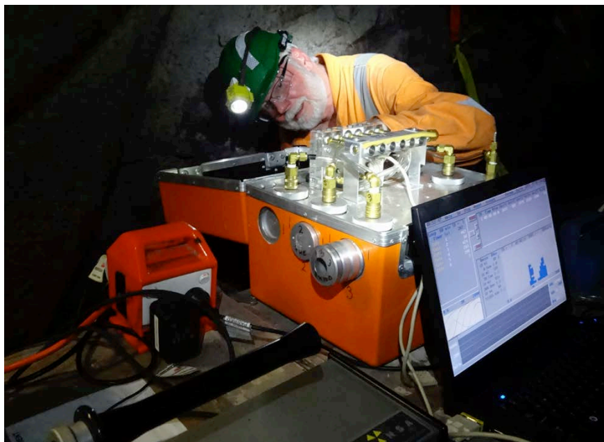
Figure 2.2 ARPANSA 6-Stage Continuous Diffusion Battery (ORANGEDB)
