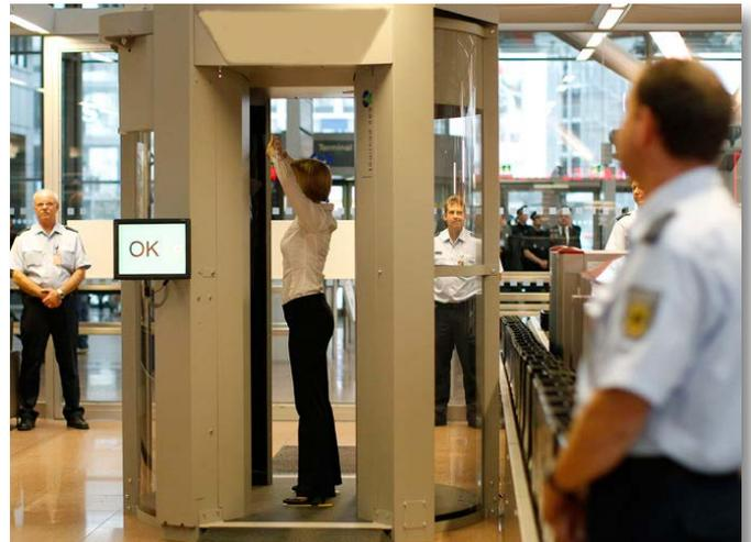
*Active millimetre wave scanner*
