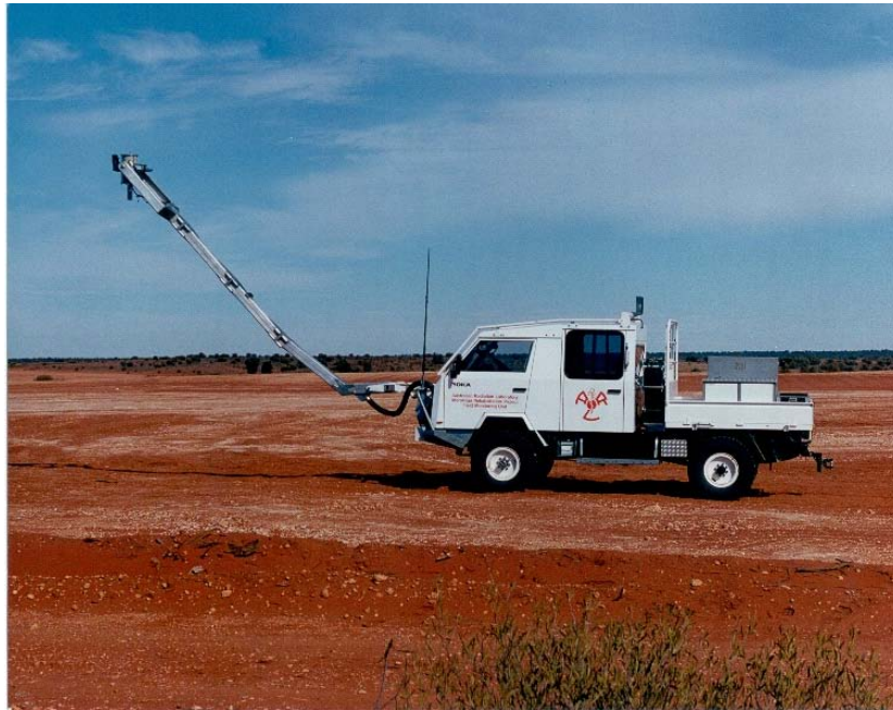
Figure 3: The purpose-built vehicle used for measurements of the areal distribution of finely divided plutonium as part of the verification studies
