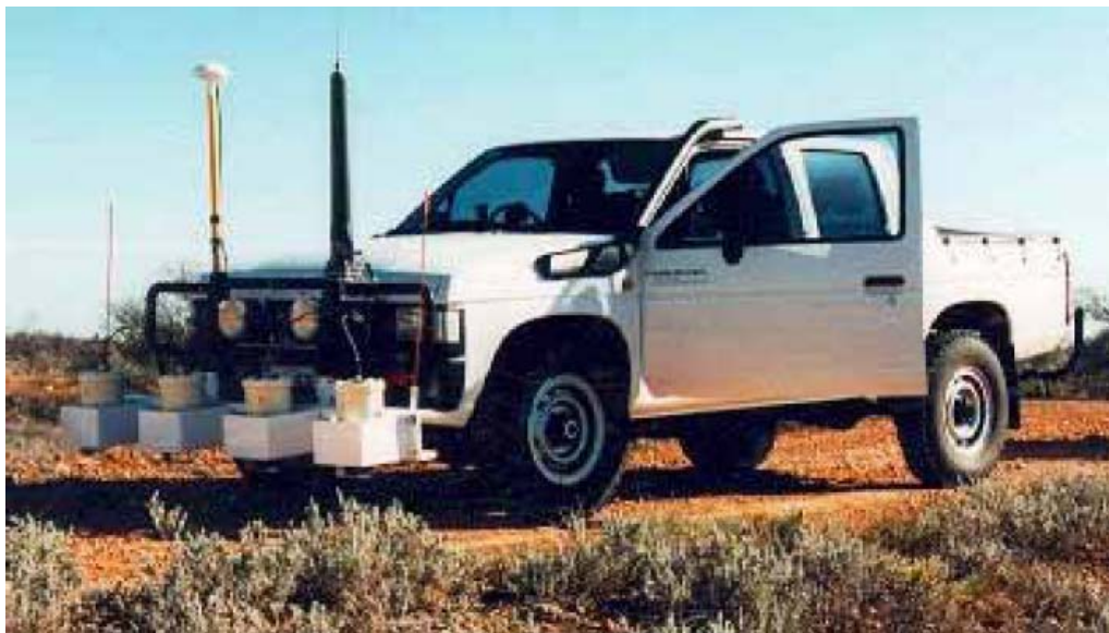
Figure 4: The purpose-built vehicle used for detection of particles contaminated with plutonium during the verification program.
